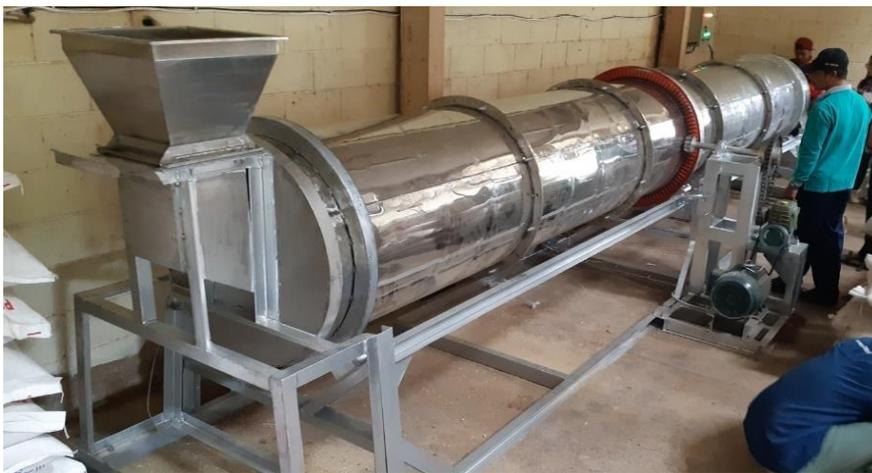
Gambar 13. Mesin Pengering Tipe *Rotary*
