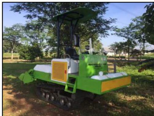
Gambar 1. Mesin Pengolah Tanah Tipe Ampibi (Rotavator)
